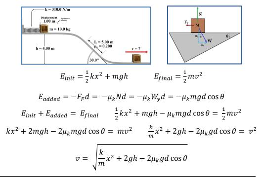
$$v = \sqrt{\frac{310\frac{N}{m}}{10.0 \, kg}} (1.00m)^2 + 2\left(9.80\frac{m}{s^2}\right) (4.00 \, m) - 2(0.200)\left(9.80\frac{m}{s^2}\right) (5.00 \, m) \cos(30^\circ) = 9.61 \, \text{m/s}$$
