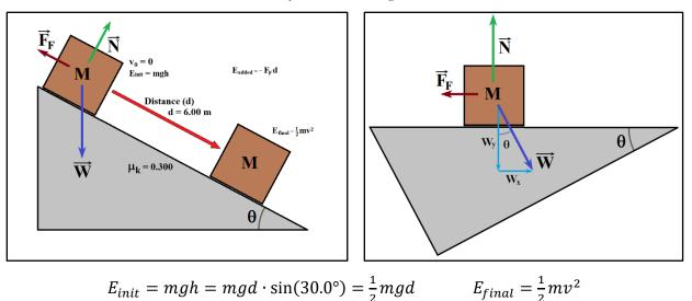
The weight (W) does work, but this is not included in  $E_{added}$  as it is already covered with potential energy. The normal force (N) doesn't do any work as it is perpendicular to the direction of motion.
