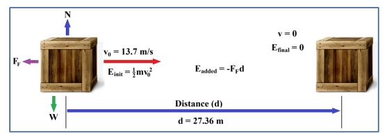
$$E_{init} = \frac{1}{2}mv_0^2 \qquad E_{final} = 0 \qquad E_{added} = -F_F d = -\mu_k N d = -\mu_k mg d$$
