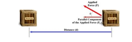
A)  $W = F_{\parallel} \cdot d = F \cdot d \cdot Cos(\theta) = (396 \text{ N})(20.2 \text{ m})Cos(30.0^{\circ}) = 6.93 \text{ kJ}$
